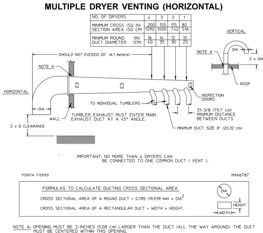
Horizontal venting **must not exceed** 20 feet (6.1 meters) - this calculation compensates for the use of a maximum of only one (1) elbow, which is the outside outlet protection.
