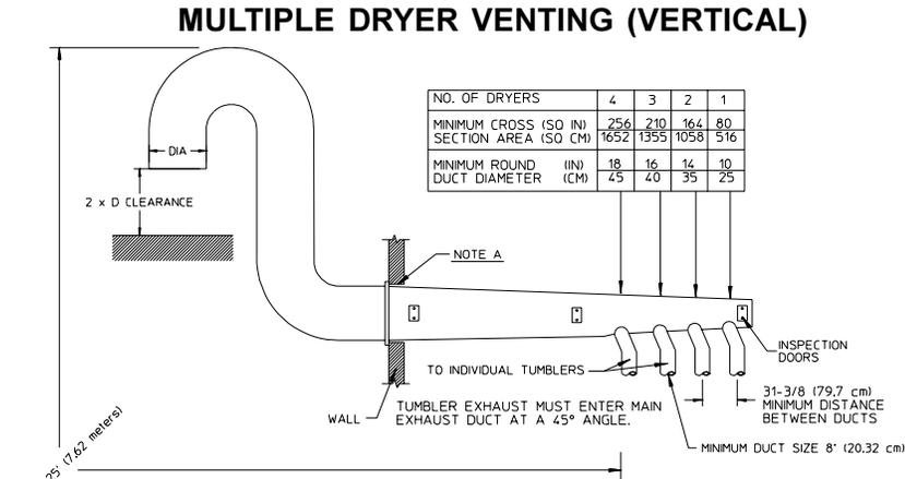
IMPORTANT: NO MORE THAN 4 DRYERS CAN BE CONNECTED TO ONE COMMON DUCT ( VENT ).
